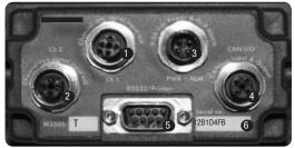
Input Channel 1, Max +/-39.0625 milli-Volts (analogue)
