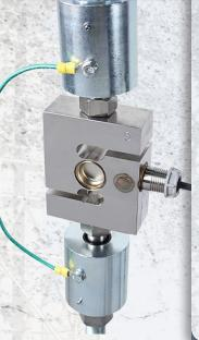
A grounding strap is attached to load cell adapters for electrical discharge protection.
