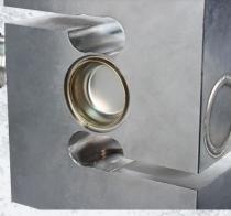
Suspension load cells are sealant potted in models ZX-250 through ZX-1000 to provide strain gauge protection against moisture, temperature, and sediment damage. Load cell models ZX-2500 and higher are cupped and welded shut for superior protection.
